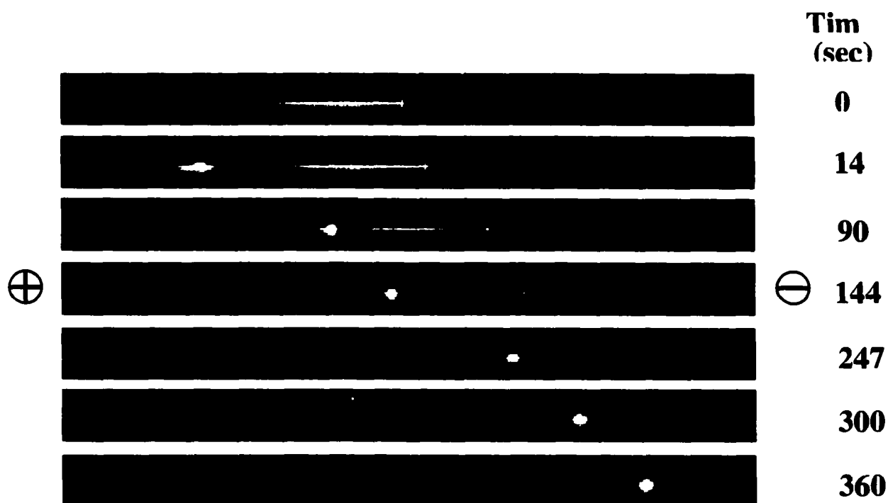
Figure 7.2. CCD pictures showing the electrophoretic movement of sperm cells inside a 10-cm long capillary detection window at different times after 22 kV voltage was applied. Notice that the sample slug had a sharp front and a dim rear before a voltage was applied. This sharp front was caused by a small air bubble, which constrained the diffusion of sperm during the process of pushing sample slug to the detection window. In this case, air bubble had no effects on the focusing process of sperm. Boar semen was diluted with BTS extender to a sperm concentration of 1.2 \times 10^7 /ml. See experimental section for other conditions.
